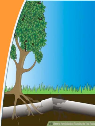
**Tree Roots**, which work their way into the sewer through joints where pipes connect.
